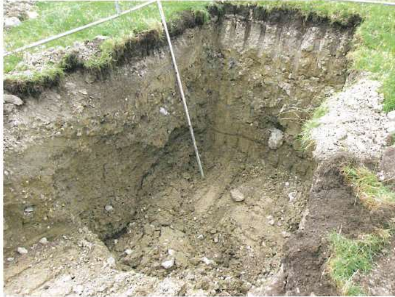
Photo showing Trial Hole
